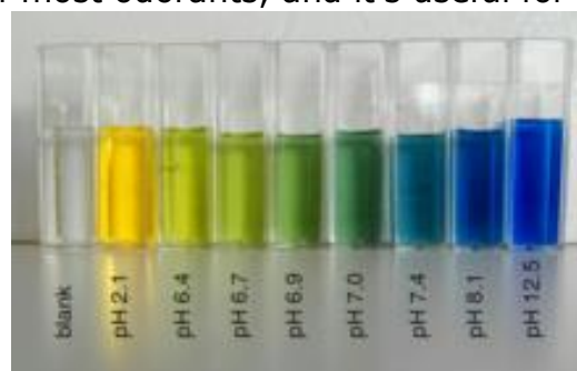
Figure 2. Bromothymol blue, an example of a color-changing pH indicator (Photo courtesy of Gregor Trefalt; Wikimedia Commons )
